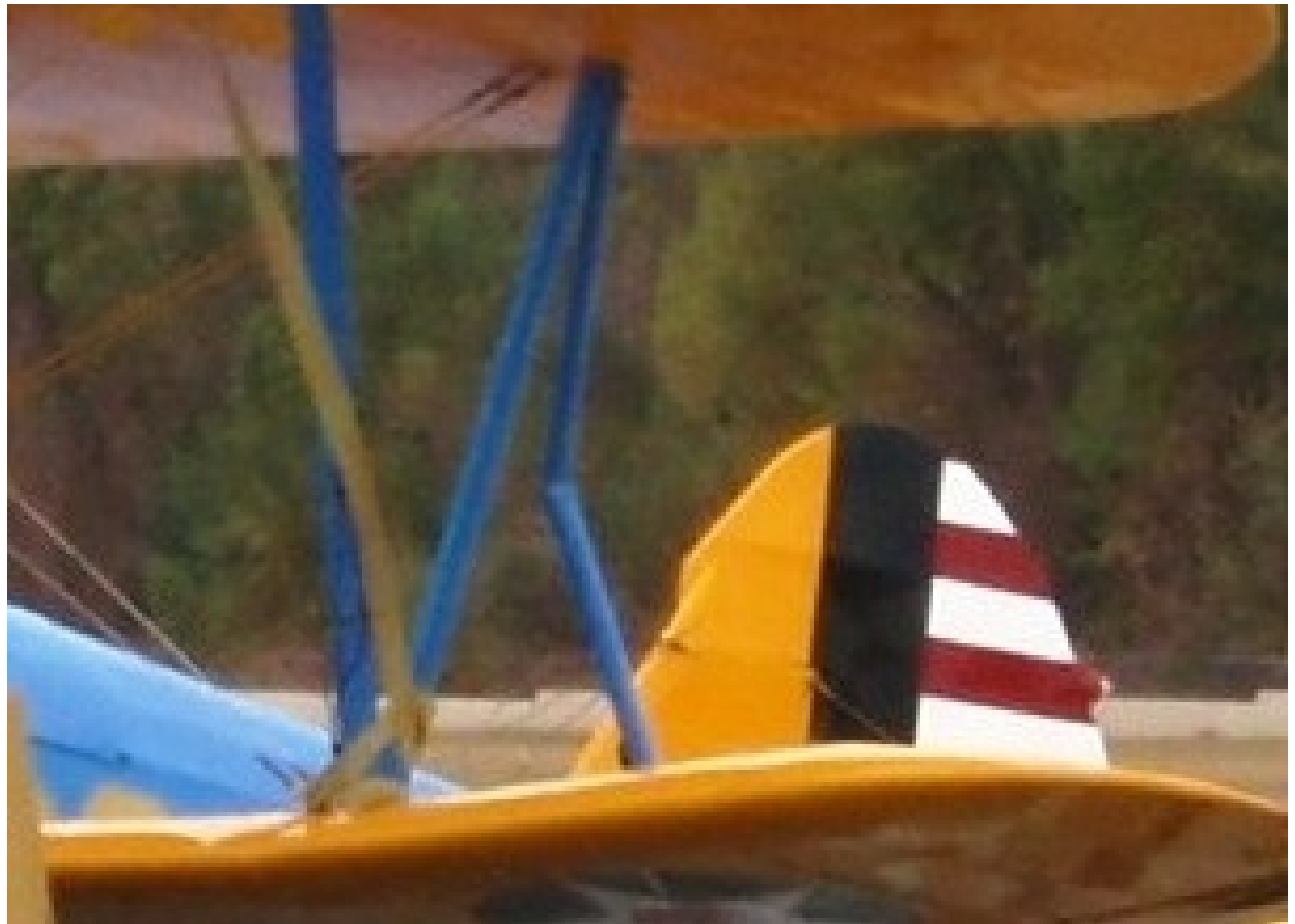
I noticed that a blue wing strut had taken so much stress that it had kinked almost halfway up
